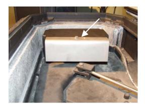
4. The hood is held in place with two bolts and nuts. To remove the bolts use a ½" socket from inside the firebox and wedge a flat blade screwdriver between the hood and the bolt head inside the top of the stove. It may be helpful to spray penetrating liquid on the nuts inside the firebox. (The nuts do not need to be replaced after the new combustor is installed, simply drop the bolts back through the hood for proper alignment).
